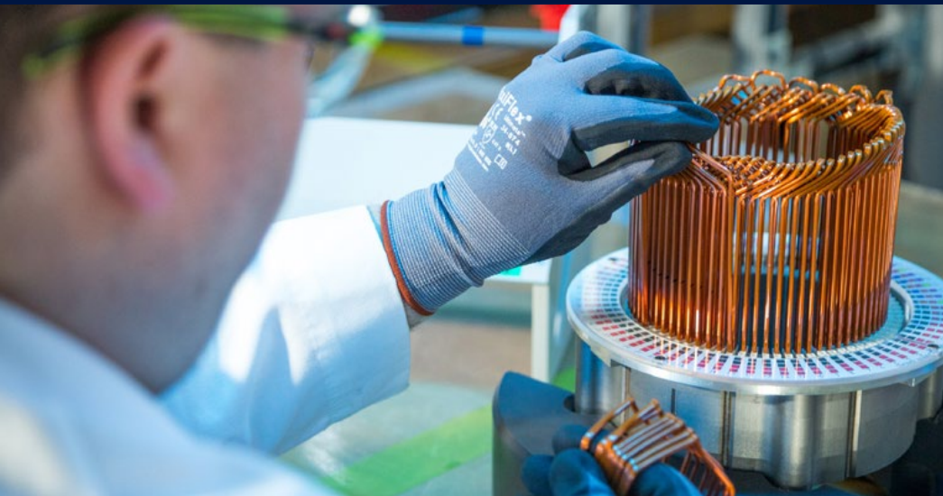
← An electric motor stator is assembled by hand during pre-production at General Motors Global Propulsion Systems Center in Pontiac, Michigan.
