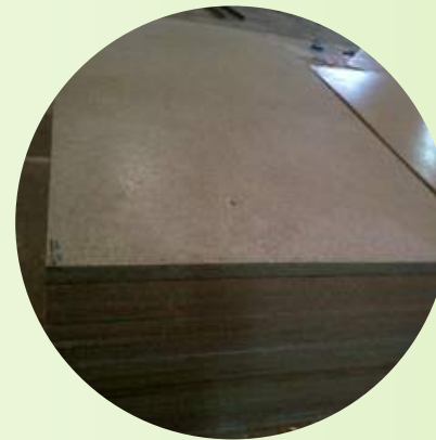
The plastic is mixed with other components, heated and pressed into building panels
