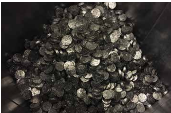
Titanium-based turnings that have been formed into briquettes
