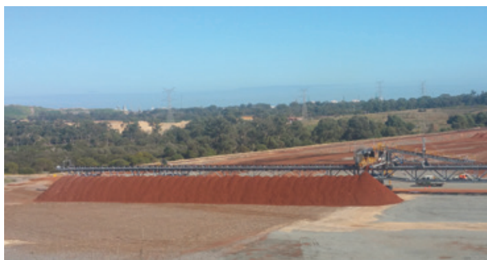
Stacking dry residue that results from the filtration process
