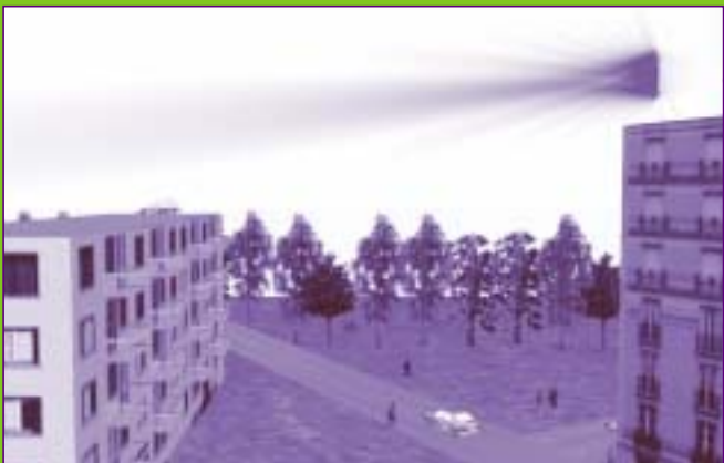
Simulation of the electromagnetic fields emitted by a GSM 900 antenna of twenty or thirty watts. The diagram shows antenna emissions following a horizontal directional schema: the exposure to electromagnetic waves is lower below the antenna than in front of it.
