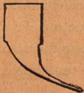
Fig. 231.—Clavo remachado, Delperier.
