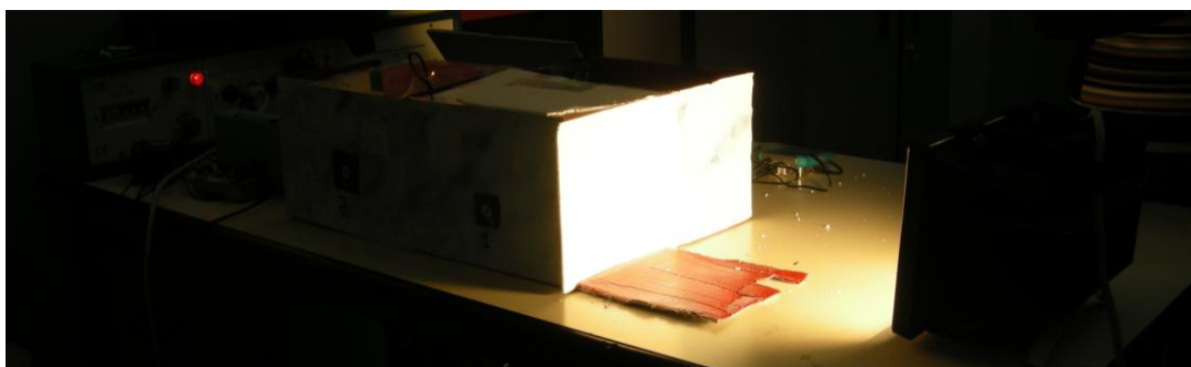
Figure 8. Test of the effect of a material during the design cycle. Room 1 is covered by a polystyrene “ceiling”, the others are uncovered. The “house” is illuminated by the 150W lamp (the “Sun”).
