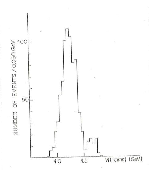
Fig. 2 :  $K^{\dagger}\pi^{\dagger}\pi^{-}$  mass spectrum for the coherent events with  $t^{+}<0.04~\text{GeV}^{2}$ . Incoherent and background events have been subtracted.
