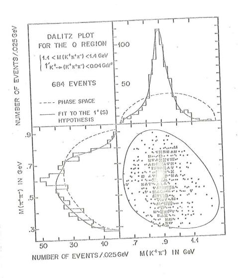
Fig. 3 : Dalitz plot for the Q events with 1.1 < M(K  $^+\pi^+\pi^-$ ) < 1.4 GeV and t  $^{'}$  < 0.04 GeV  $^2$
