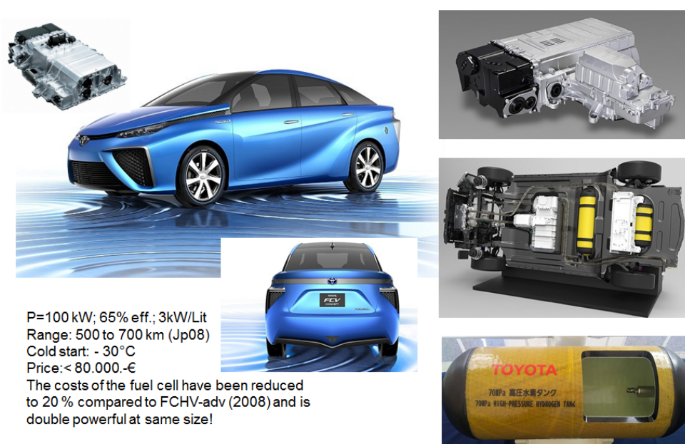
Figure 13: Toyota "MIRAI" (=Future) vehicle and FC components
