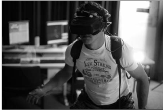
Figure 2. Image of a participant wearing a HMD. Note the straps of the back pack that house the control box. This control box in turn is connected by a long DVI cable to the computer rendering the images and interfacing with the tracking system.
