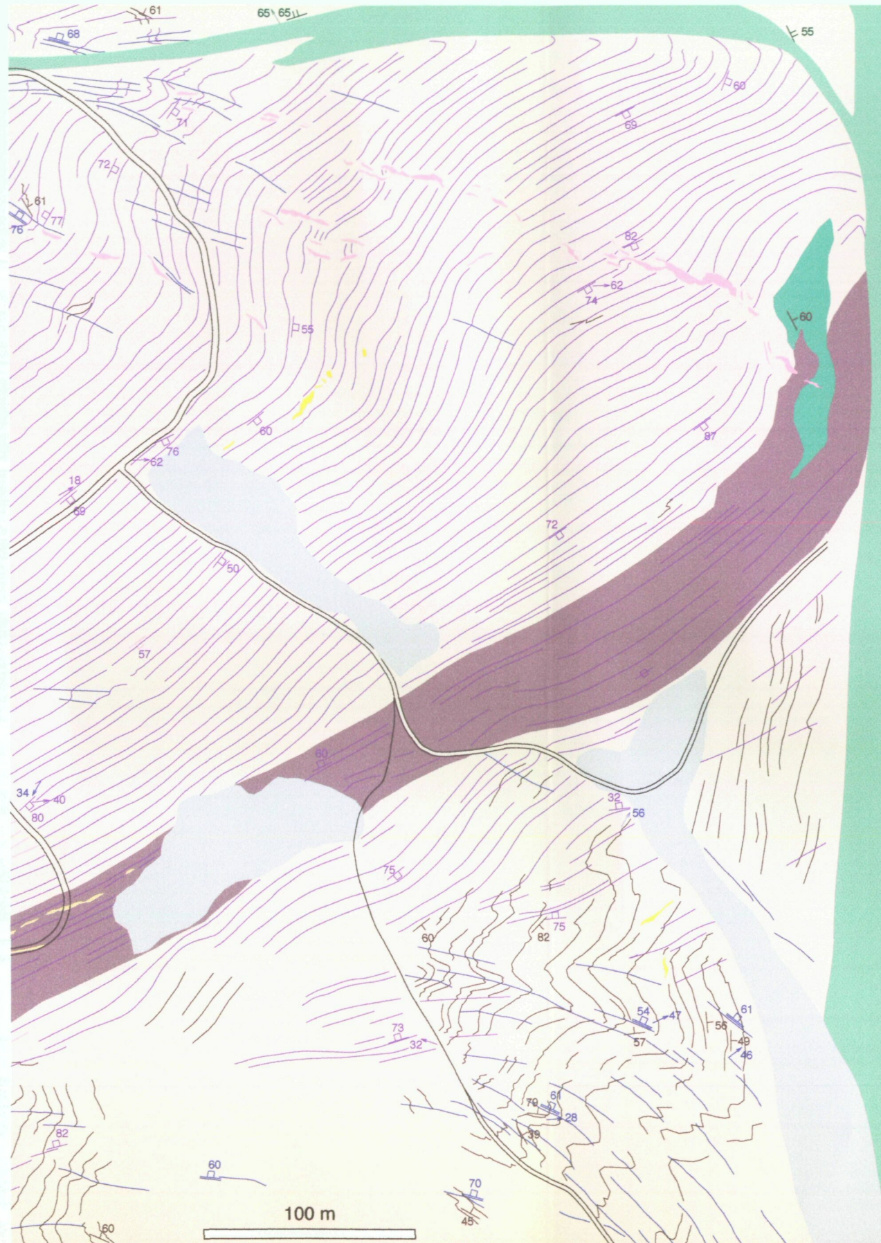
Fig. 44. Structural map of La Birba road zone and equal area lower hemisphere projections of main structural elements of two differentiated sub-areas (NW and SE). In sub-area SE, S 1 is the dominant foliation and it is folded mainly by D 3 . S 3 axial planar foliation is more intense than S 2 . Sub-area NW is a D 2 high strain domain. S 2 replaces S 1 as the dominant foliation. It is slightly folded by D 3 .
