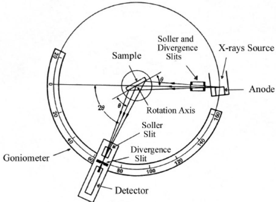
**Figure 2.4:** Schematic picture of a x-ray diffractometer
