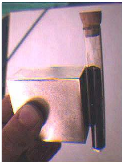
Fig. 1. Example of a magnetic aerogel attracted by a NdFeB magnet. The aerogel correspond to sample A3 (see text).
