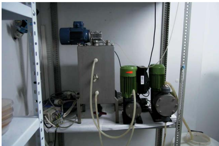
Figure 7.1. Pilot plant used to enrich the EBPR population and to perform the AnOx experiments.
