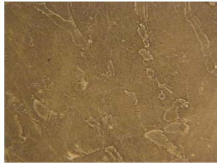
a) Implanté room temperature – recuit 1650°C N<sub>2</sub>
