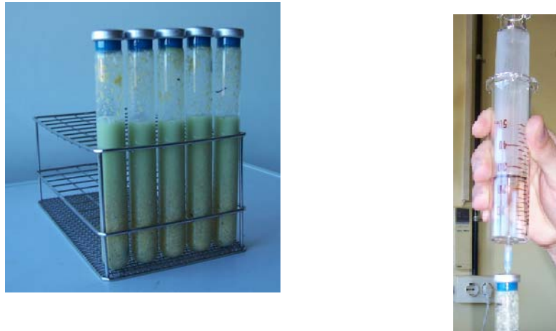
Figure 7.1. Tubes containing the media (left). Measuring the accumulated gas (right).
