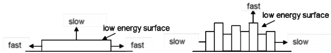
Fig. 3-10 Schematic indicating the transition from thermodynamically preferred c_{\perp} growth to kinetically preferred a_{\perp} growth at high supersaturation [135].
