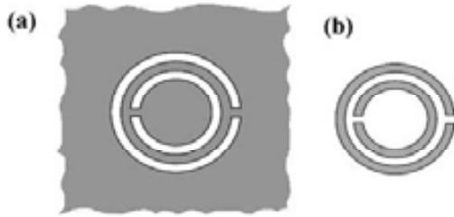
Fig. 1 Topology of the circular CSRR (a) and SRR (b). Metal regions are depicted in gray. Square-shaped or rectangular geometries are also possible
