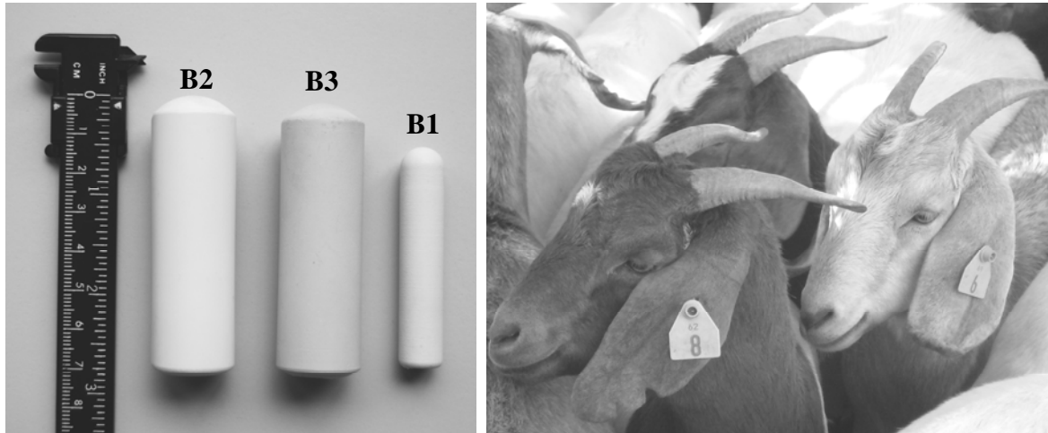
Figure 4.1. Electronic rumen boluses and visual ear tags used.
