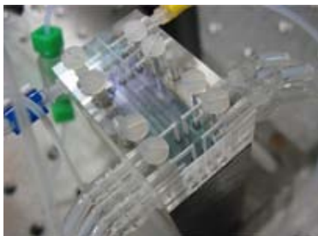
Figure 6.5: Complete fluidic platform picture, with external PMMA housing, connections and integrated polymeric microfluidics layer.
