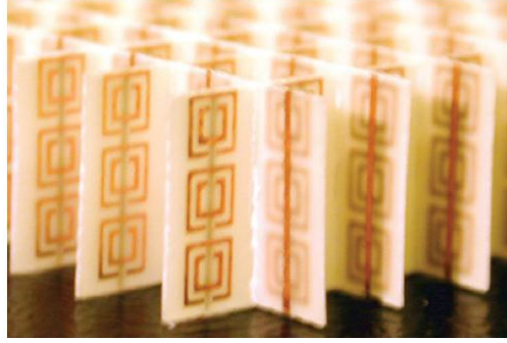
Figure 2.5. Photograph of the first 2D left-handed structure used to demonstrate the negative refraction, extracted from [56].
