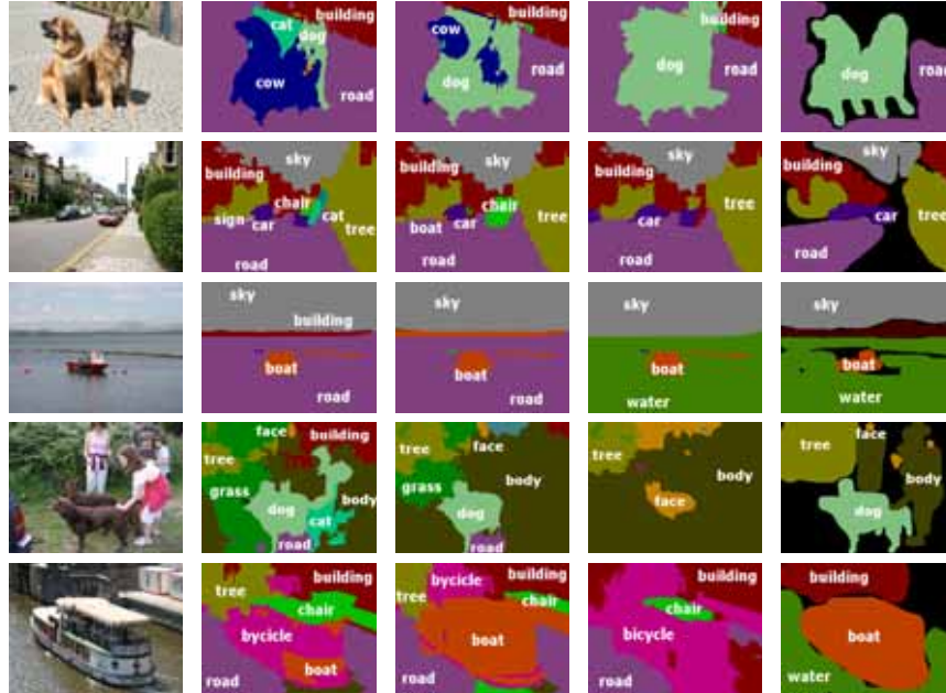
Figure 4.8: Qualitative results for the MSRC-21 dataset. Comparison between (b) no consistency potentials, (c) robust P^N -based potentials, and (d) harmony potentials. (e) Ground-truth images. In the first three rows the harmony potential successfully improves segmentation results. The last two rows show failure cases of harmony potentials.
