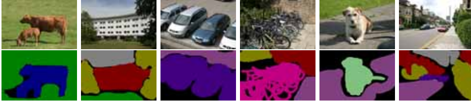
Figure 3.1: Images and their ground-truth segmentations. Images extracted from the MSRC-21 Dataset, which show the kind of segmentation that we desire.
