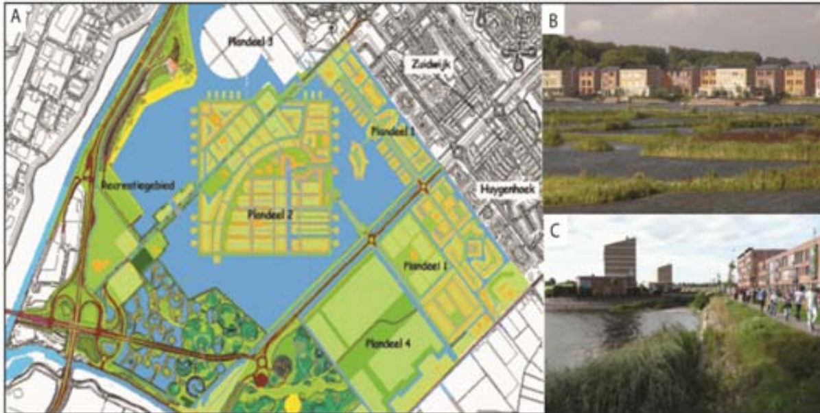
Figure 2.12: A) Site plan of the City of the Sun. (Hoogheemraadschap Hollands Noorderkwartier, 2005). B) Constructed wetlands of the City of the Sun “lunapark” used both for intensive purification of surface water and recreational uses (Schuetze, 2010). C) Clearly visible in the urban design with water the sufficient freeboard for the fluctuation of the water level in the city of the Sun. (Schuetze, 2010)
