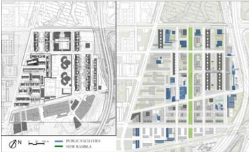
Figure 4.6. Urban structure of La mina before (left) and after (right) renewal.
