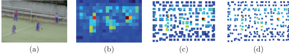
Figure 5.1: Coarse-to-fine inference. We propose a method for the fast inference of multi-resolution part based models. (a) example detections; (b) scores obtained by matching the lowest resolution part (root filter) at all image locations; (c) scores obtained by matching the intermediate resolution parts, only at location selected based on the response of the root part; (d) scores obtained by matching the high resolution parts, only at locations selected based on the intermediate resolution scores. A white space indicates that the part is not matched at a certain image location, resulting in a computational saving. The saving increases with the resolution .
