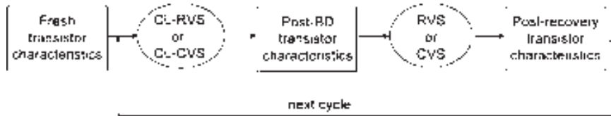
Fig. 1. Measurement sequence designed to analyze the dielectric BD reversibility. To limit the current during the CL stresses (CL-RVS or CL-CVS), the compliance of the measurement equipment was used.
