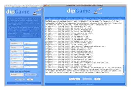
Figure 6.14: Screenshot of the GameManager. On the left side of the figure you can see the main window of the game manager where the game can be set. When running the game, the window on the right side of the figure pops up providing real-time results of the game execution.
