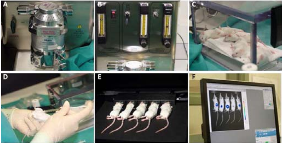
Figure 30. In vivo BLI imaging using the IVIS System. A-C. Mice were anesthetized using 2% isoflurane into the induction chamber. D-E. Before imaging, mice were given an intraperitoneal (i.p.) injection (150 mg/ kg body weight) of D-Luciferin substrate, placed into the IVIS Instrument and maintained under anaesthesia. F. The IVIS® Spectrum was used for the time-course of the in vivo BLI of mice. Mice were imaged once weekly beginning on day 0 after tumour inoculation to evaluate and quantify the bone tumour growth until the end of the experiment 7 weeks after cell inoculation.
