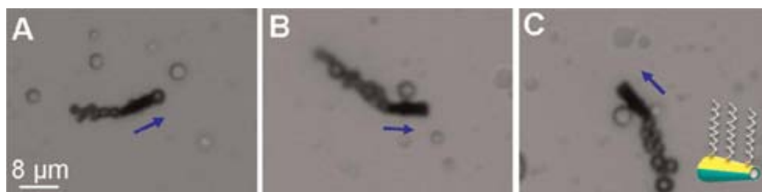
Figure 5. SAM-modified micromotor carrying floating droplets of motor oil in a fuel-enhanced oil-contaminated water sample. Images taken after 78 s navigation in the fuel-enhanced solution (conditions, as in Figure 2). (A, B, C) Time-lapse images showing the microsubmarine approaching, contacting, and carrying the droplets, respectively. Inset: Cartoon of the dodecanethiol-modified micromotor. Arrows indicate the direction of the micromotor movement.
