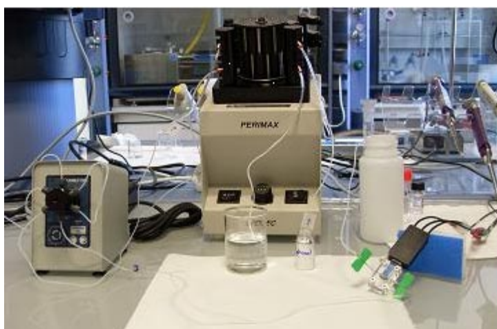
Figure 9. FIA setup based on home-made flow-through cell, peristaltic pump (Perimax16/3) and a model Ch-Instrument potentiostat 660A electrochemical workstation from CH Instruments Inc., Austin, TX.
