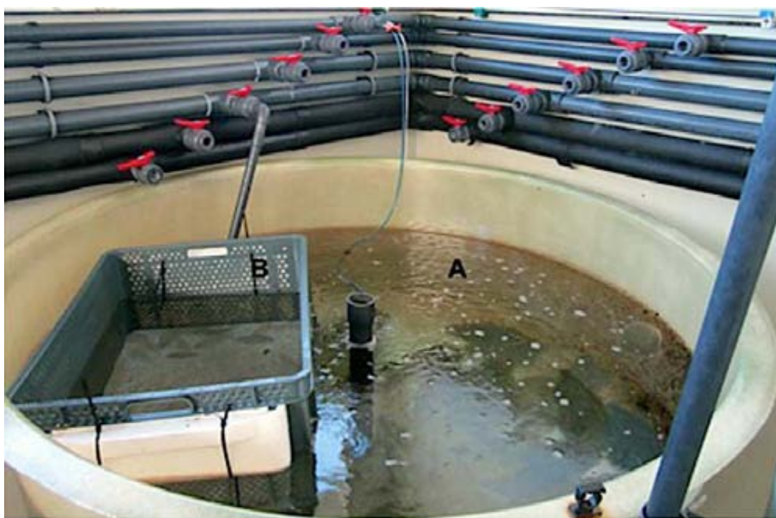
Figure. 7.2: Fiberglass 1,500 litres cylindro-conical tank containing donor fish (A), with a smaller (400 litres) quadrangular floating fiberglass tank containing receptor fish (B) during experimental infections.
