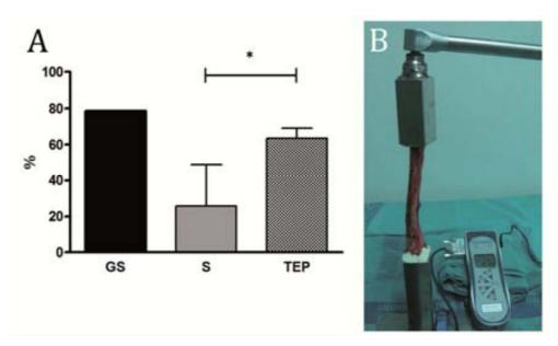
**Fig. 4-11.** Biomechanic test. A) Biomechanical strength percentage of the treated tibiae relative to contralateral tibiae. GS: Gold Standard (black), S: Scaffold (gray), TEP: Tissue engineered product (black and white). B) Image of the biomechanical torsion test performed. \* Significant differences (p<0.1).
