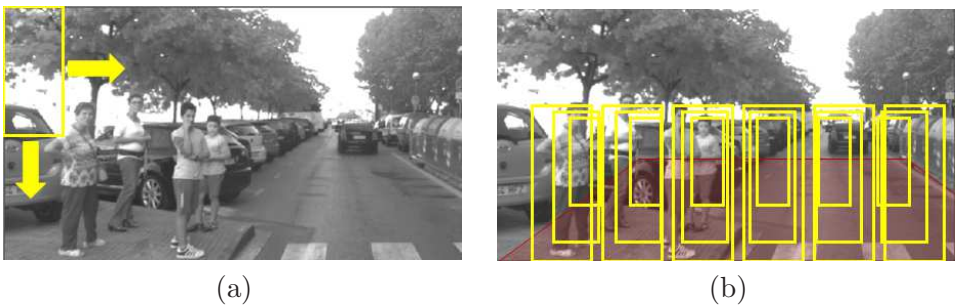
Figure 2.2: Basic candidate generation methods for pedestrian description. (a) sliding window, and (b) linear to road approach.
