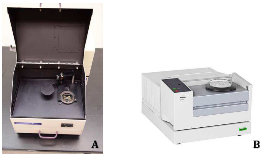
Fig10.Solid sample accessories from the NIR used A) RCA from Foss NIR Systems and B) petri dish sample holder from Buchi
