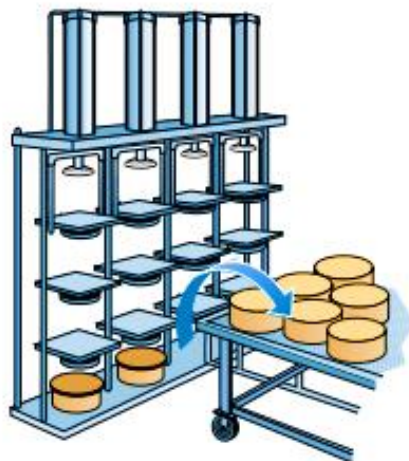
Fig. 2.25. Vertical pressing unit with pneumatically operated pressing plates. Reproduced from Bylund (2003) .
