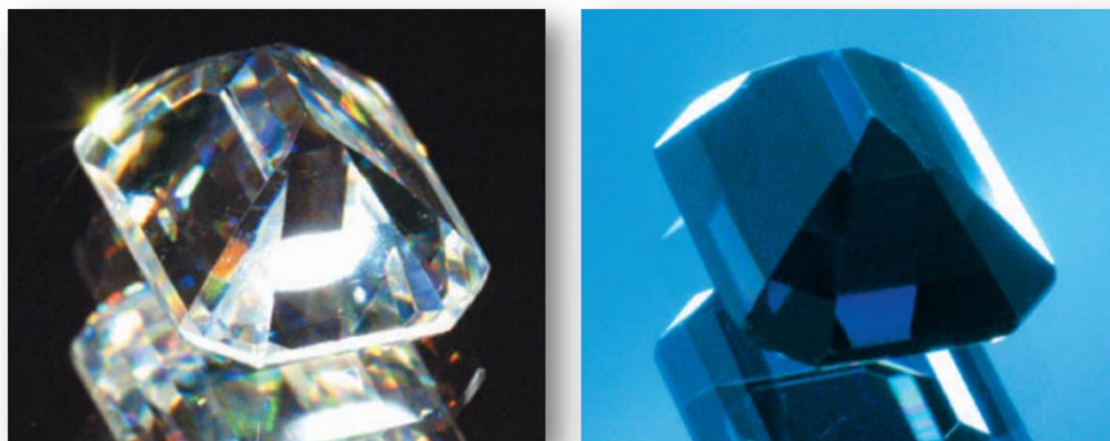
Figure 1.12 STO cut and polished as diamond (left), the same crystal after reduction (right) – the removal of oxygen atoms from the surface makes it conductive and thus opaque. Pictures taken from [83].
