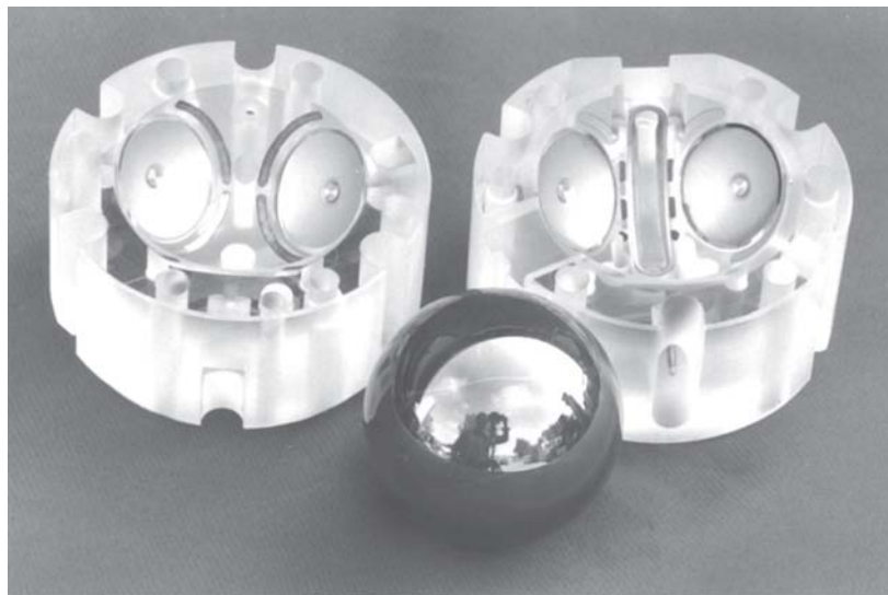
FIGURE 5.6: Photograph of an actual GP-B gyro and its housing.
