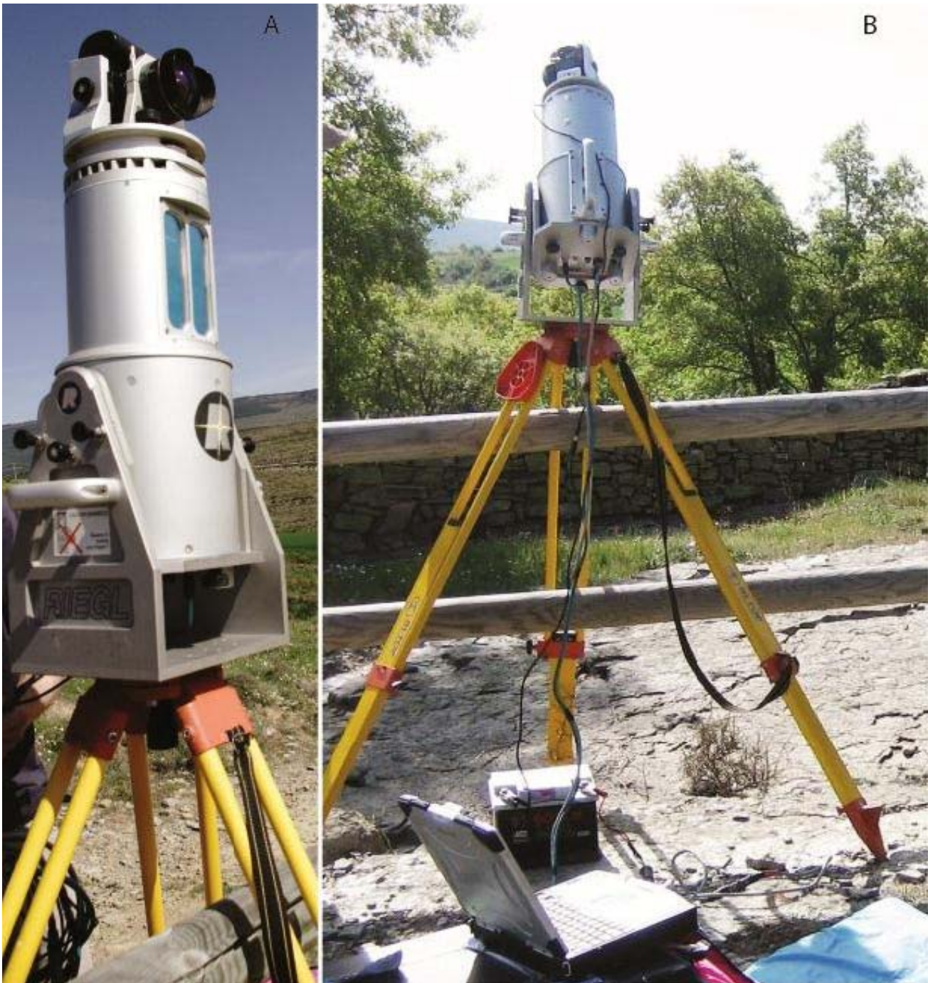
Figure 2.7. Close-up of the LiDAR methods with details of the portable RIEGL LMS-Z420i 3-D laser scanner and the attached camera (6.1 megapixel Nikon D100) (A); LiDAR functioning in the field while scanning the El Frontal tracksite (B).
