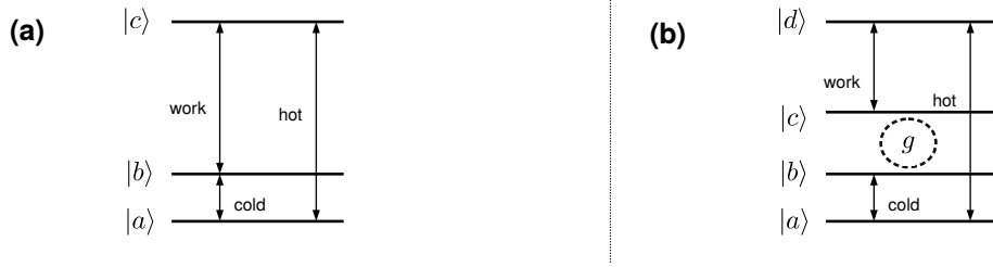
FIGURE 6.4: Schematic illustration of (a) a three-level heat pump and (b) a four-level irreversible device. The three external heat baths ('work', 'hot' and 'cold') have temperatures T_w > T_h > T_c . The arrows indicate dissipative coupling between a given heat bath and the corresponding transition. The internal parameter g in the four-level device controls its 'degree of irreversibility' (see text for details).
