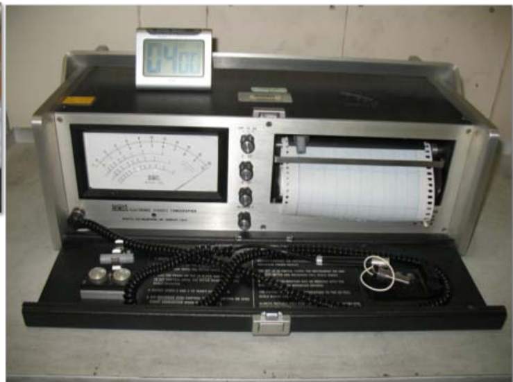
Figure 16 & 17: The Schiøtz tonographer (model 720; Berkeley Bioengineering, Inc., San Leandro, CA) used in this study (left). Mr KS Lim performing tonography to one of the participants (right).
