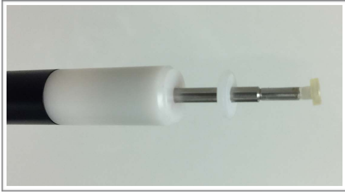
Figure 5. Pneumatic tonometer or pneumotonometer used in this study to measure the IOP without fluorescein. (Model 30 Classic; Reichert Ophthalmic Instruments, Depew, NY).
