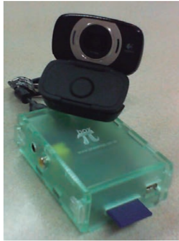
Figure 5.1 – Our hardware setup for the cheap eye-tracker prototype.
