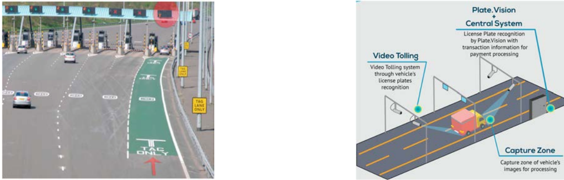
Figure 2.4: Traditional electronic tolling systems: (Left) DSRC [M6t03] and (right) ANPR [Vis17].
