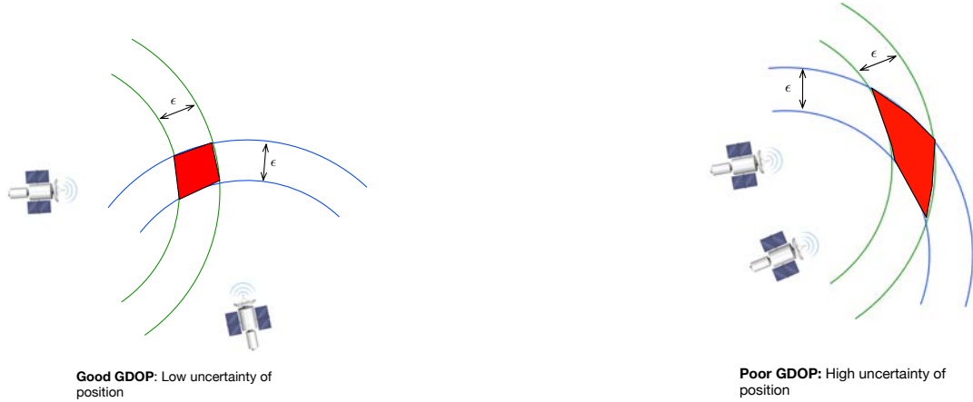
Figure 3.10: Example of position estimation with range measurements and the quality of the position estimate for different satellite geometries.
