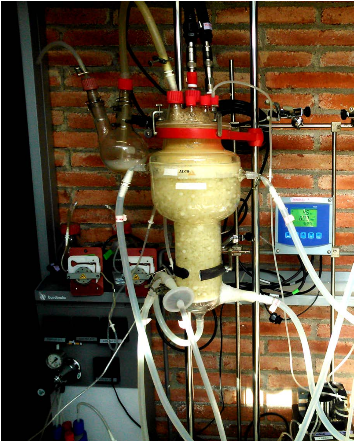
Figure 3.1: One of the 2 L air-pulsed bioreactors used in this thesis.
