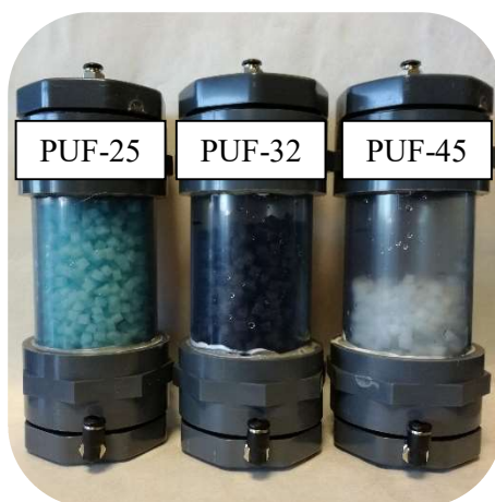
Figure 8.2. Pictures of the 3 polyurethane foam (PUF) with different densities with the 65-mL fermentation media in the reactor.
