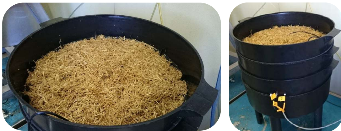
Figure 6.3. Pictures of the 40-L packed-bed bioreactor filled with a solid mixture based on winterization oil cake and sugar beet molasses blended with wheat straw.
