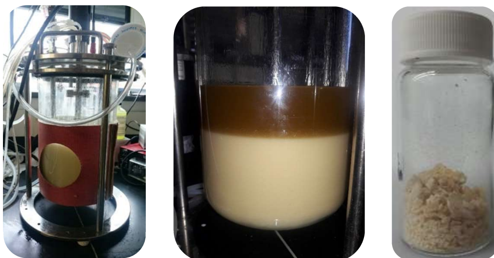
Figure 7.8. Pictures of the bioreactor during the fermentation (left), when the fermentation was stopped (center), and the SLs extracted (right).
