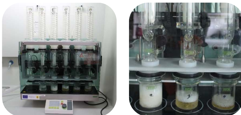
Figure 3.13. Pictures of the Soxhlet E-816 (Büchi) during the extraction of fats.
