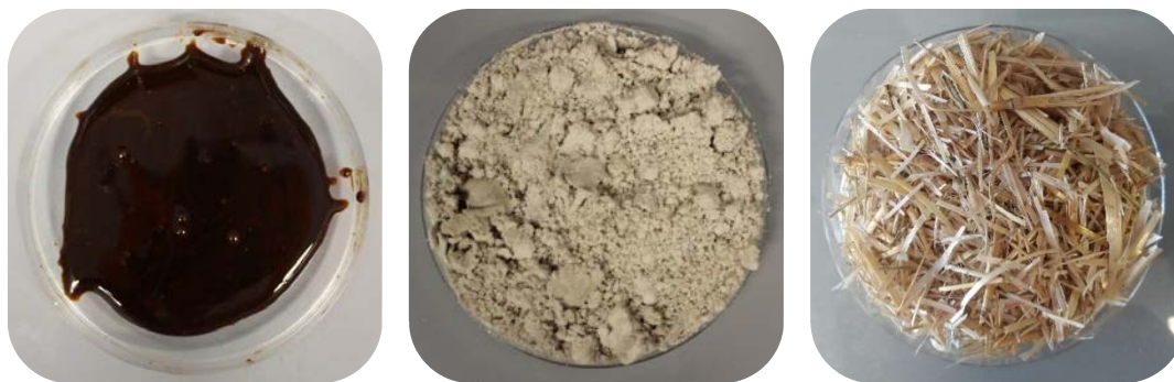
Figure 5.1. Physical appearance of the sugar beet molasses (left), the winterization oil cake (center), and the wheat straw (right).
