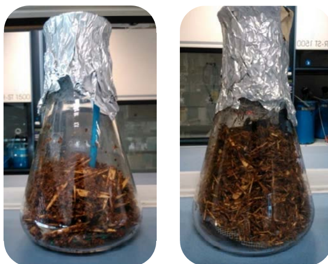
Figure 4.14. SSF mixtures based on MOL and WOC blended with wheat bran (left) or wheat straw (right).
