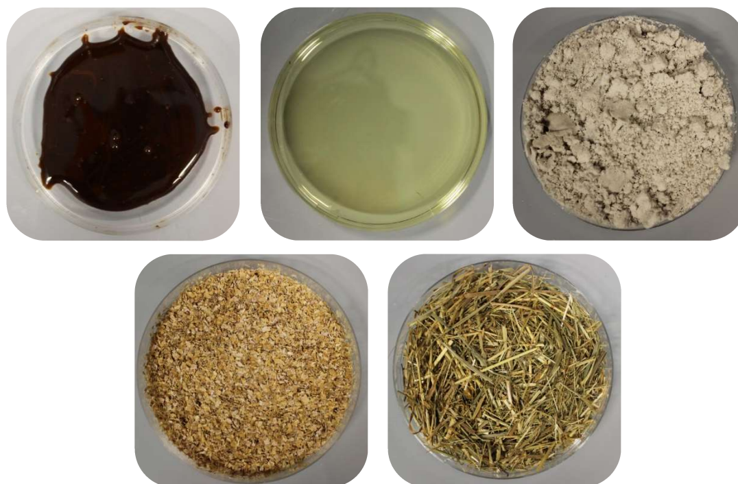
Figure 4.1. Physical appearance of the sugar beet molasses (up left), waste cooking oil (up center), winterization oil cake (up right), wheat bran (down left) and wheat straw (down right).
