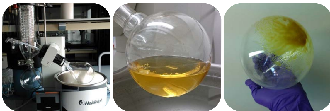
Figure 3.12. Pictures of the rotary evaporator (left), a round bottom flask during the evaporation of the ethyl acetate (center), and the SLs (right).
