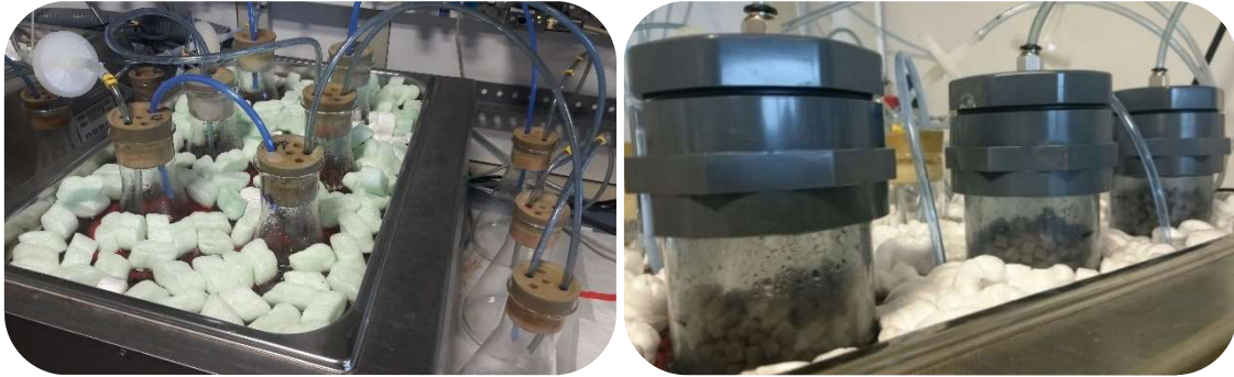
Figure 3.6. Pictures of the Fermentation System I when the reactor is a 0.5-L Erlenmeyer Flask (left) or a 450-mL cylindrical polypropylene packed-bed reactor (right).
