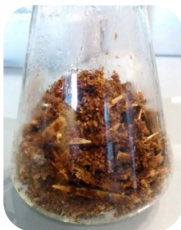
Figure 4.4. SSF mixture based on glucose and oleic acid blended with wheat bran.
