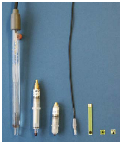
Figure 3.5 | Miniaturization of potentiometric pH sensors. On the left-hand side a commercial pH sensor with diameter 12 mm (commercial standard) is shown; the next three sensors are made by conventional techniques; the three sensors on the right-hand side are fabricated by printing techniques. Source: [10].
