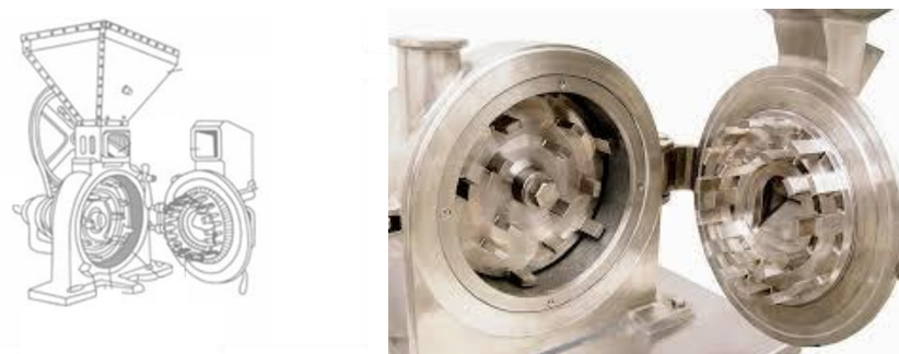
Fig. 1.5 The schematic diagram and object picture of the impact column mill
