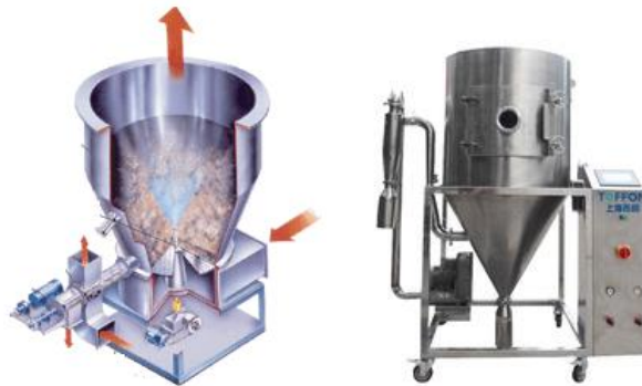
Fig. 1.18 The schematic diagram and object picture of spray granulation
