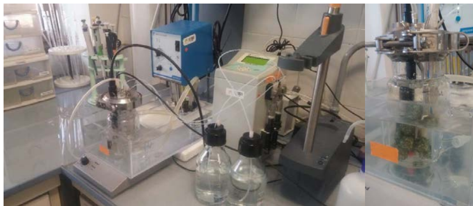
Figure 3.12: A picture of the respirometer at UAB laboratories and detail of the 0.3 L vessel filled with immobilised PUF cubes.
