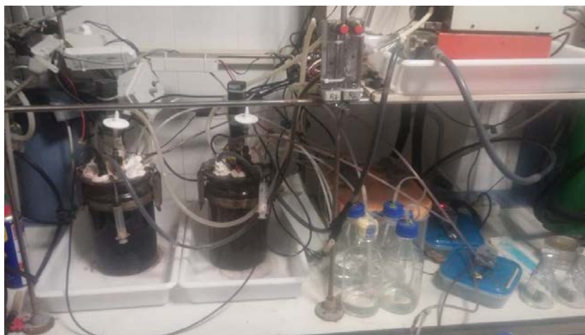
Figure 3.8: The UAB experimental set-up consisted of two rotating, submerged, packed bed reactors.
