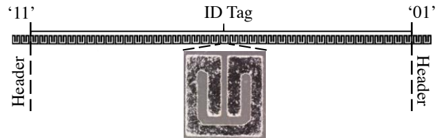
Fig. 7. Photograph of the tag with all bits set to '1' printed on din A4 paper.
