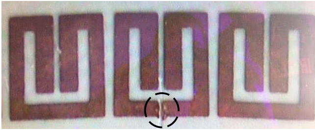
Fig. 13. Photograph of the detuned SRR.
