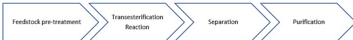
Figure 8.15. Schematic process for industrial biodiesel production.
