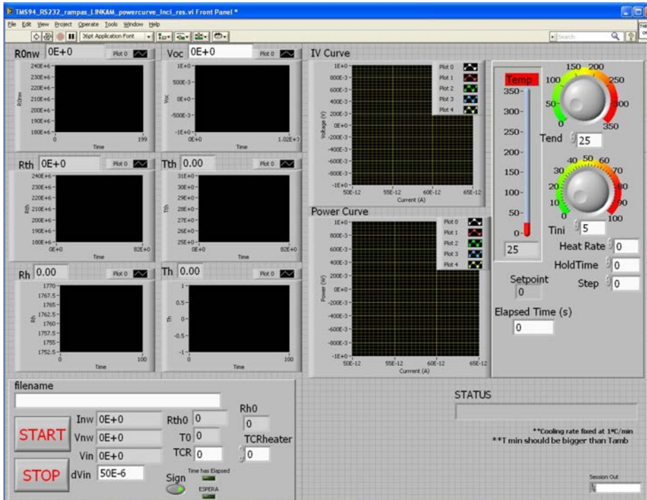
Figure 2.13: LabVIEW program developed for thermoelectric power measurements. Measurements of hot side and cold side temperatures and NW resistance can also be performed simultaneously.
