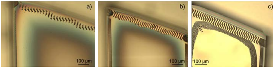
Figure 3.14: Optical images of different stages of KOH etch. a) Under-etched device, there are still Si bulk connections under the membrane. b) Properly etched device, membrane is completely released. c) Over-etched device, KOH started to etch device Si of SOI.
