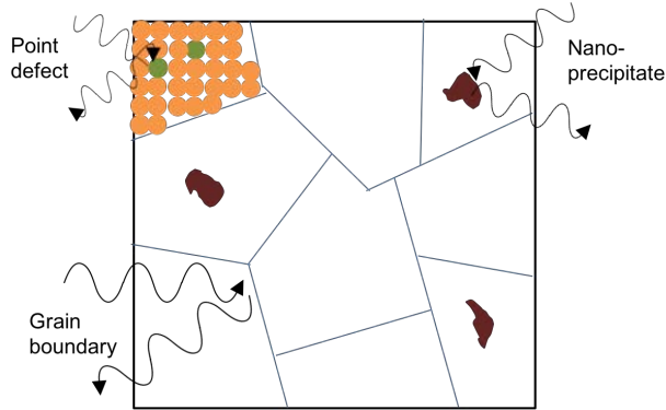
Figure 1.5: Some of the different phonon scattering mechanisms. Adapted from [25].
