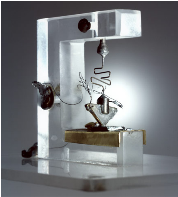
FIGURE 1.1: Replica of the first transistor designed in the Bell labs by Bardeen, Brattain and Shockley in 1947.
