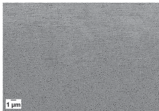
Fig. 2. PS spheres of 200 nm diameter assembled onto Au substrate via electrophoretic deposition.
